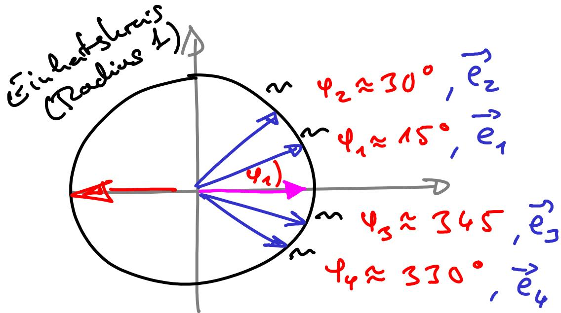
$$\overline{\varphi} = \frac{\varphi_1 + \varphi_2 + \varphi_3 + \varphi_4}{4} ??? = 180^\circ$$
