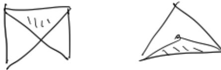
Abbildung 80: not a triangulation <sup>81</sup>
