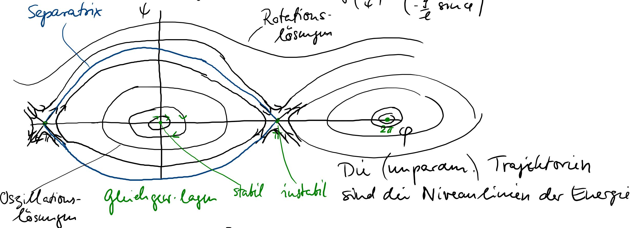
$$E(\varphi, \dot{\varphi}) = \frac{m}{2} l^2 \dot{\varphi}^2 - m g l \cos \varphi$$
