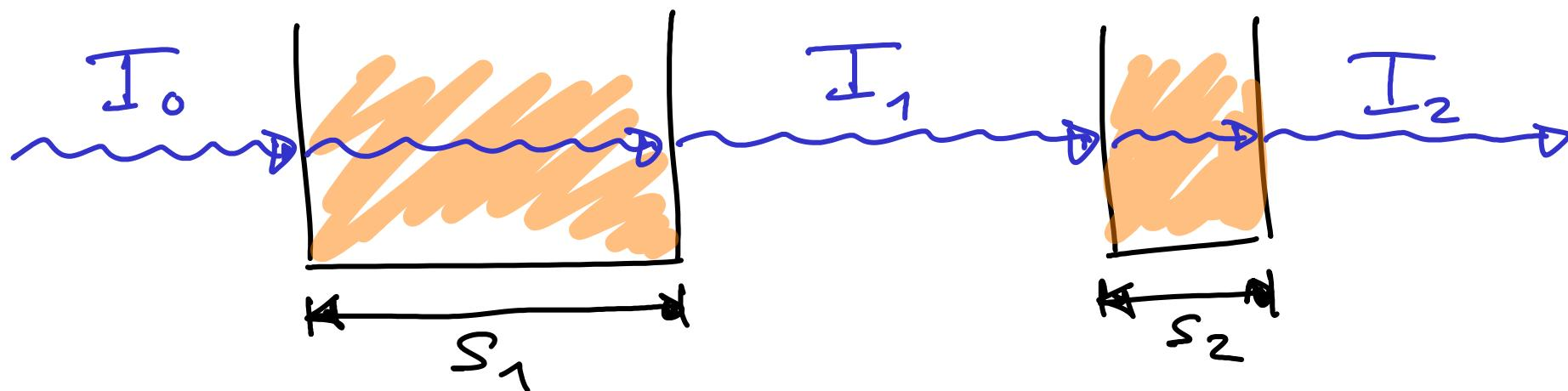
$$I_1 = \alpha_{S_1} I_0, \quad I_2 = \alpha_{S_2} I_1 = \alpha_{S_1} \cdot \alpha_{S_2} \cdot I_0$$
