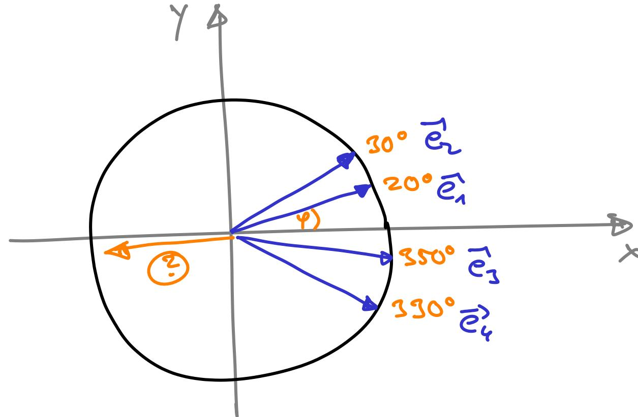
$$\bar{\varphi} = \frac{20^\circ + 30^\circ + 350^\circ + 330^\circ}{4} = 182,5^\circ$$
